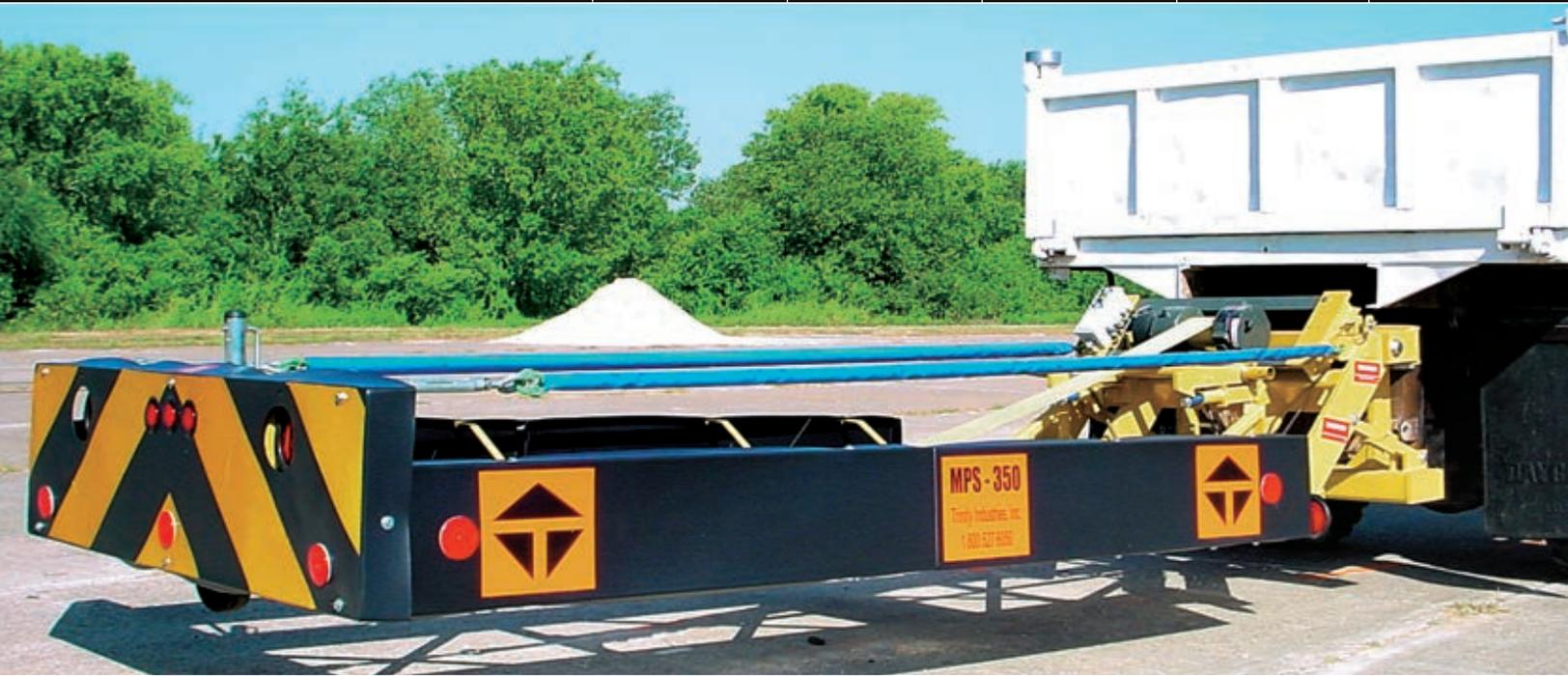
The MPS-350™ (Mobile Protection System 350™) is available for use on stationary or moving shadow or support vehicles and is the first truck-mounted attenuator to pass NCHRP report 350 Test Level 3. It has an open design and all-steel construction of functional components. The MPS-350™ design is a new concept that eliminates bulky crushable cartridges.
